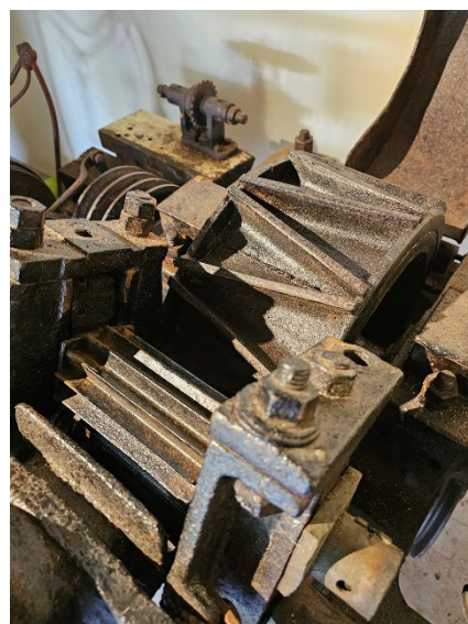
Image 5 An open view of the rotor, beater bar and feed rollers. Courtesy of Templeton Flax Museum
